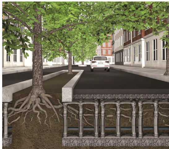
Silva cells are installed under other infrastructure and support the paved surfaces while providing space for planted trees' roots to grow and expand.
